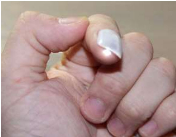
HandSight micro-camera built into a false finger nail along with a tiny LED light.
